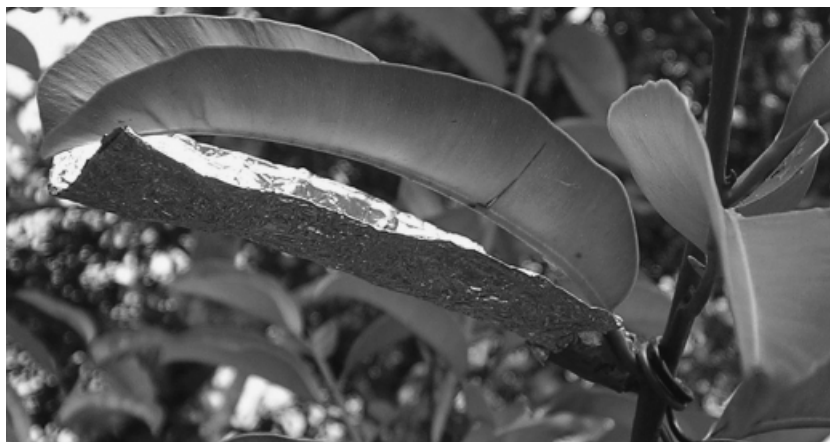
FIGURE 1. A leaf warmed by a resistance heater in a heating experiment conducted at Floresta Nacional do Tapajos, Brazil. Each heater added 1.2 W of energy to the leaf and was affixed several centimeters below the leaf. Heaters warmed the leaves continuously through the experiment.
